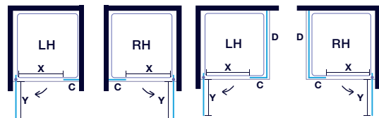
Pivot Door & Inline Panel in Recess Pivot Door & Inline Panel with Side Panel
